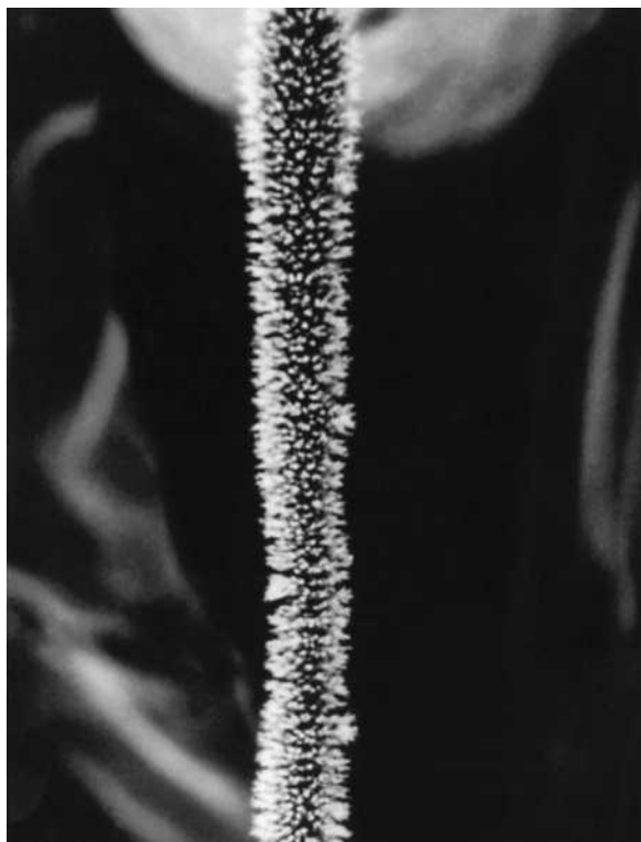
FIGURE 20-5 Photomicrograph of a carbon microneedle emitter. (Courtesy of R. P. Lattimer, BF Goodrich Research and Development Center.)
