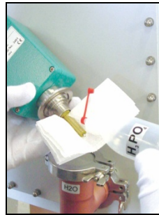
8. Moisten winding with phosphoric acid.
