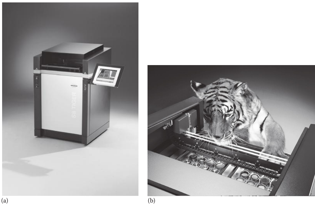
Figure 8.44 (a) The S8 TIGER, a floor-mounted commercial WDXRF system. (b) The sample compartment of the S8 TIGER, showing the multiposition autosampler with typical samples such as polished metal flats on the left and pressed pellets on the right. (The namesake operator shown is not standard! Geaux Tigers!) © 2013 Bruker, Inc. www.bruker.com. Used with permission.)
