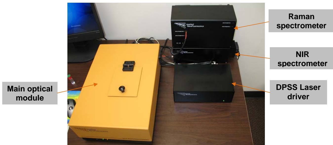
Fig. 1. NS2 modules (control computer is not shown).
