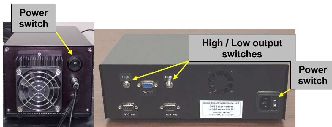
Fig. 3. Back panels of the NIR Spectrometer module (left) and DPSS Laser Driver module (right). On the DPSS Laser Driver, the high / low output toggle switches should remain in the up (High) position except during alignment or service.
