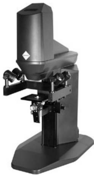
Figure 15 Spectral Dimensions Model Sapphire, NIR Chemical Imaging system for measuring NIR microscopic images.
