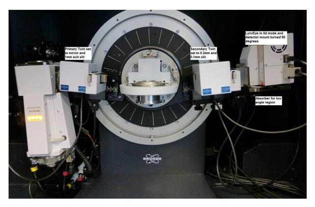
The NIST SRM2000 standard sample was mounted on a height adjustable clay slide sample holder.
