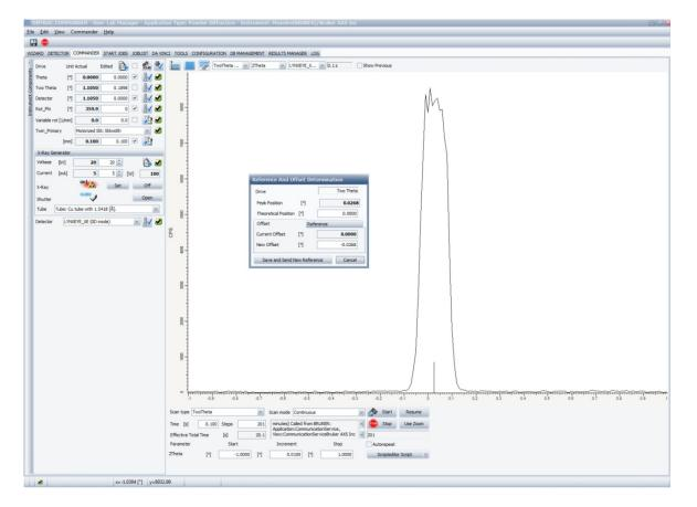
If the peak is too high as in the screenshot above, tighten the screw below the assembly and loosen the top screw slightly.
