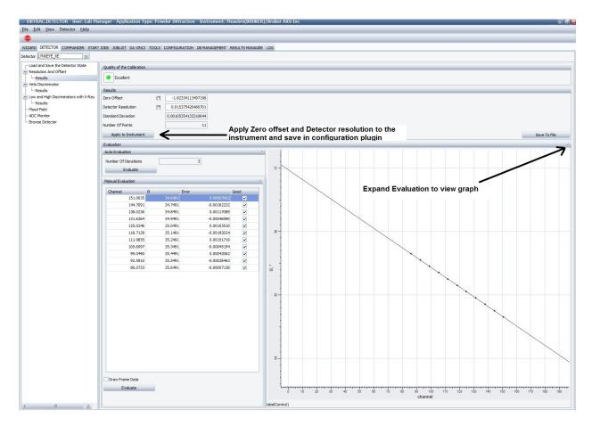
After the calibration run the results should indicate excellent quality. Apply the determined Zero Offset and resolution values to the configuration plugin. There is no download necessary.
