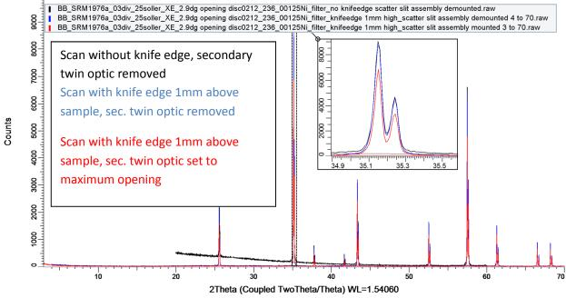
Typical measurement ranges for pharmaceutical samples range from 3 to 40° 2theta and for mineral samples from 3 to 70° 2theta. These ranges can be measured with the full opening of the LynxEye detector using all channels. The background from air scatter can be controlled by using the knife edge above the sample as well the secondary twin optic.
