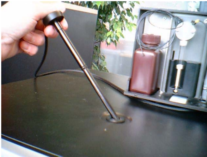
Picture 2-1: Inserting the injector carrier into the injector port
