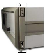
4. Make sure, that the guide rails are assembled in the 19" rack to avoid damage when mounting the instrument into the rack.
