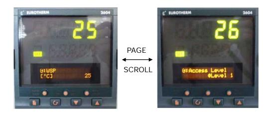
Using the "DOWN" key you can select the "Config" menu. After entering the password, modifications are possible for authorized personnel only! To get back to the parameter-menue press the PAGE key and SCROLL key together.
