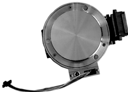
Figure 232-2 TipView Adapter Ring for AFM or LFM microscopes
