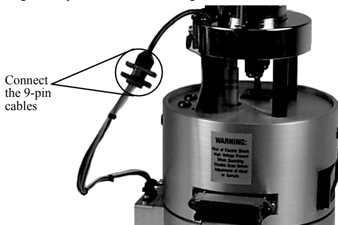
Figure 232-5 Connect the scanner to the TipView adapter ring through the 9-pin cable.
