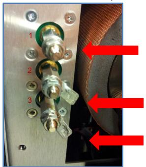
Remove the two white heater wires with the Ring Connectors to terminal post #1 and two white heater wires with Push on Connectors to terminal posts #2 and #3
