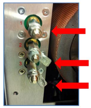
Attach the two white heater wires with the Ring Connectors to terminal post #1
