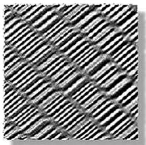
Figure 5-6. MFM image showing the magnetic signature of data bits written on a hard disk, 3 \mu m scan.
