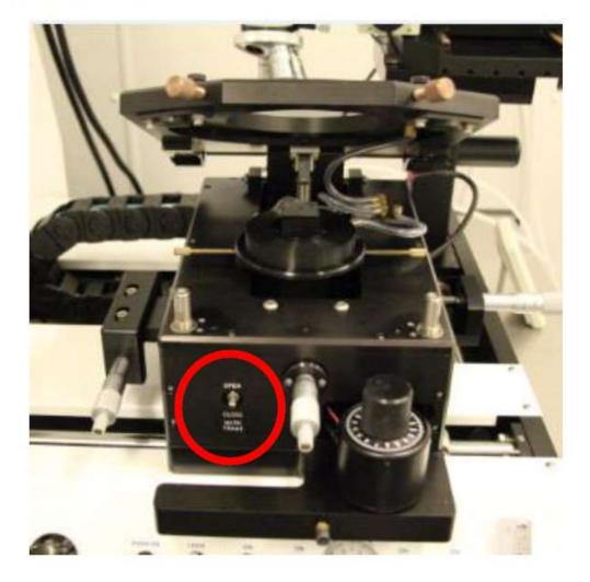
8. Load your sample. BEFORE CLOSING THE MASK FRAME MAKE SURE THAT THE MASK FRAME WILL NOT TOUCH YOUR SAMPLE. ADJUST Z IF YOU ARE NOT SURE.
