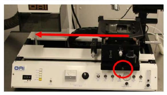
13. When the exposition is finished. Bring back the chart and unload your sample following the steps in this order: Adjsut Z, stop sub vac, open frame, unload sample
