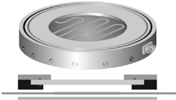
FIGURE 9.20 Schematic view of the Planartron ® source. The antenna structure is placed under a quartz plate. This arrangement is especially designed for use in Plasmodul ® [40].
