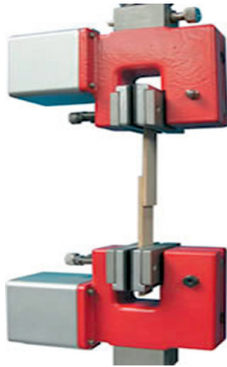
FIGURE 9.10 Lap joint shear test specimen in a tester device.
