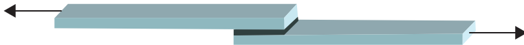
FIGURE 9.9 Schematic of adherends (blue) and Adhesive layer (black) in Single-lap Joint Shear Test (per ASTM methods D1002 for metal/metal, D3164 for plastic/metal and D3163 for plastic/plastic adherends).
