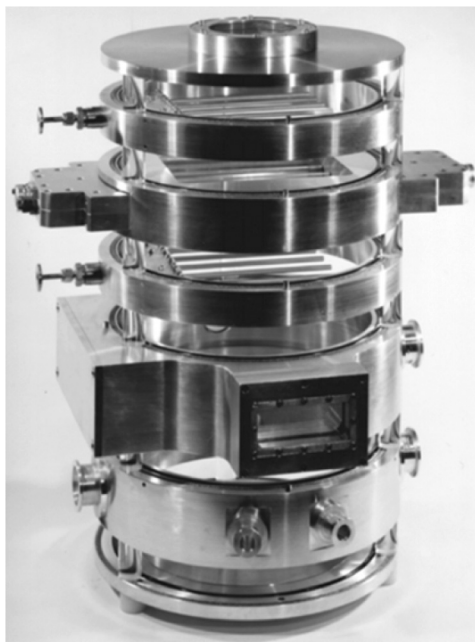
FIGURE 9.18 Plasmodul ® device with gas inlet system, plasma source, reaction chamber, and diagnostic ports [40].
