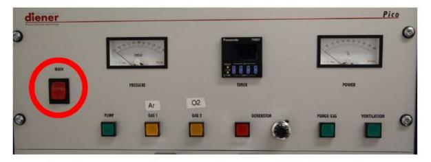
3. Place the sample in the chamber and start the pump. Wait for the pressure to be below 0.4 mbar
