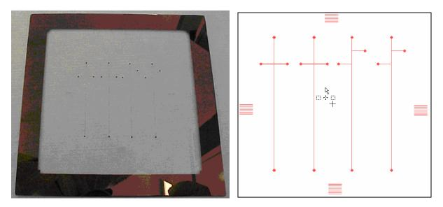
The mask that will be used to fabricated the microfluidic devices was created with the Heidelberg DWL-200 Laser Pattern Generator and L-EDIT V10.01. The microfluidics are designed within a 3.25" diameter so that the master integrates with the master holder. The mask has two standard microfluidic designs with 50um wide channels and windows for alignment with a 4" silicon wafer.
