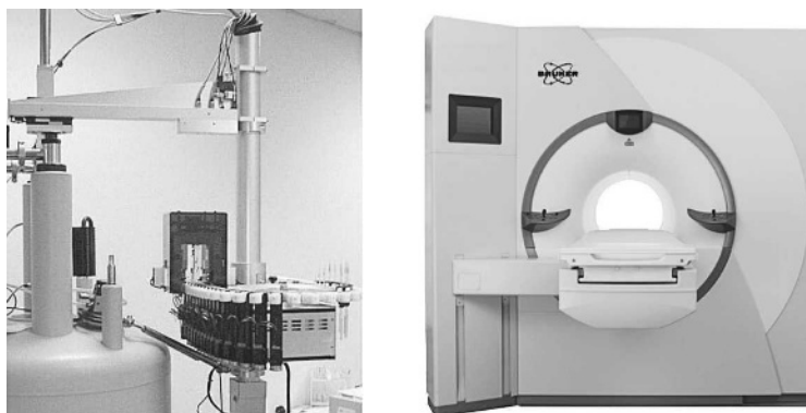
Figure 15.25 Sample introduction for NMR spectrometers. Left, automatic introduction of a sample placed in an ‘NMR tube’ within the magnetic field produced by a superconducting coil maintained at liquid helium temperature (reproduced courtesy of Varian). Right, a large magnet employed for the introduction of a particular kind of sample – the human body (part of a MRI instrument from SMIS).
