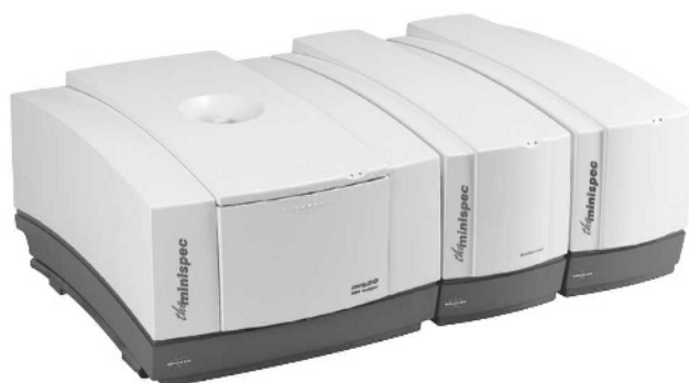
Figure 15.32 Low resolution ^1\text{H} NMR instrument for routine analyses. The analyser operates on the principle of pulsed NMR and is used for quantifying water and fat in numerous food products (model minispec, reproduced courtesy of Bruker).
