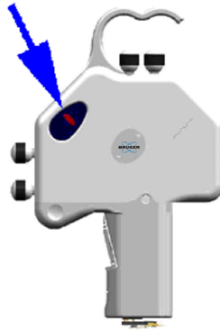
Figure 10.1f Coarse alignment should leave the laser spot in the center of the indicator.
