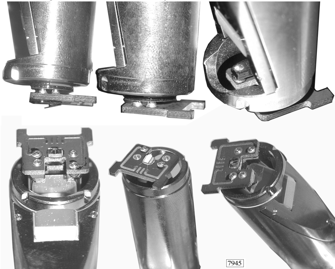
Figure 7.3c Six Views of an Active Tip Probe Mounted on a Dimension Scanner
