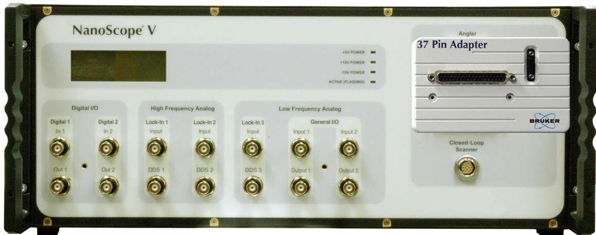
Figure 4.3b 37 Pin Adapter plugged into the NanoScope V Controller
