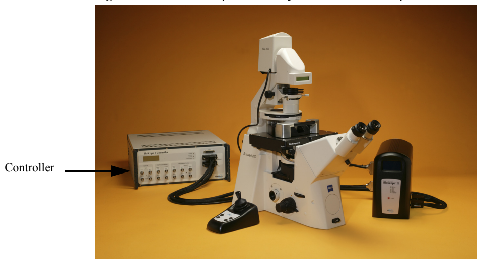
Figure 1.1b A BioScope II SPM System with NanoScope V Controller
