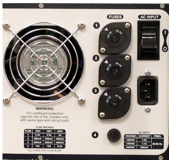
Figure 11.1b Fuse Holders on the Back of the NanoScope V Controller
