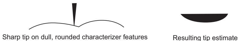
Figure 6.6d A Sample with No Sharp Features Yields a Dull Tip Estimate
