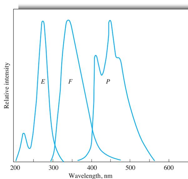
FIGURE 15-5 Spectra for tryptophan: *E*, excitation; *F*, fluorescence; *P*, phosphorescence. (Adapted from G. G. Guilbault, *Practical Fluorescence*, New York: Marcel Dekker, 1973, p. 164. Courtesy of Marcel Dekker, Inc.)
