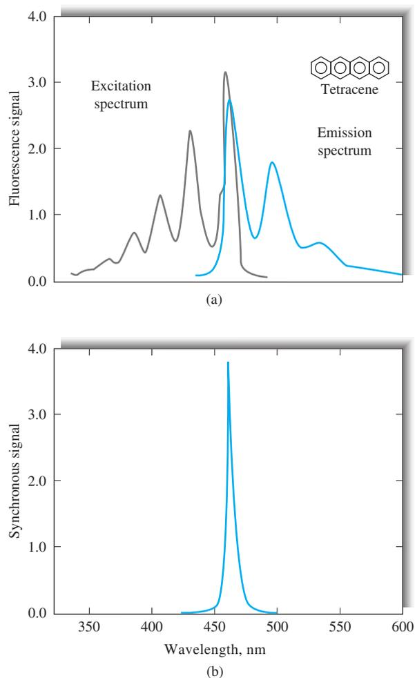
**FIGURE 15-7** Synchronous fluorescence spectra. In (a), the excitation and emission spectra of tetracene are shown. In (b), the synchronous spectrum is shown for a fixed-wavelength difference of 3 nm. (From T. Vo-Dinh, *Anal. Chem.*, **1978**, *50*, 396, DOI: 10.1021/ac50025a010. Figure 1, p. 397. Copyright 1978 American Chemical Society.)
