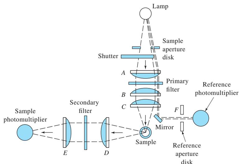
**FIGURE 15-10** A typical fluorometer. (Courtesy of Farrand Optical Components and Instruments Division of Ruhle Companies, Inc.)
