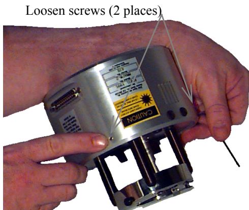
Figure 205-5 Loosen screws on the edge of the MultiMode base to separate the motor plate from the housing.
