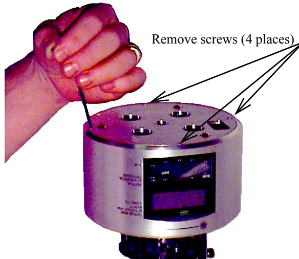
Figure 205-1 Remove four screws securing the bottom plate to the base.
