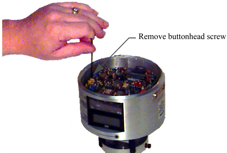
Figure 205-2 Remove the button head screw securing the main board to the base (above).
