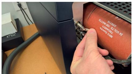
3. Measure the resistance. There are two heater circuits. I measured resistances of 9.3 - 9.4 ohms on both heater circuits in my shop unit. Any other pair should give infinite resistance (make sure if you are making the connection by using your fingers to hold the meter probes against the connectors, that you are not measuring your body resistance!)
