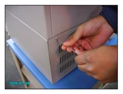
2. Find out the main circuit where the fuse locates and then, uninstall the fuse.
