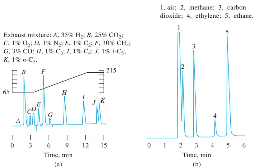
**FIGURE 27-22** Typical gas-solid chromatographic separations: (a) a 5 ft.  $\times$  1/8 in. molecular sieve column; (b) a 30 m  $\times$  0.53 mm PLOT column. C<sub>n</sub> = hydrocarbon with *n* carbons.
