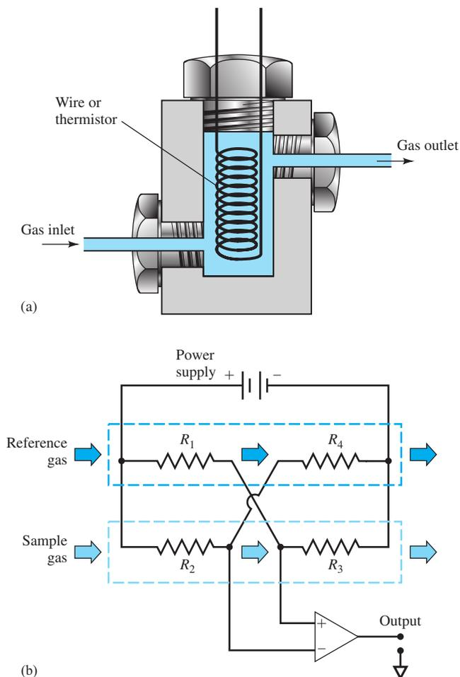
**FIGURE 27-10** Schematic of (a) a thermal conductivity detector cell and (b) an arrangement of two sample detector cells ( $R_2$  and  $R_3$ ) and two reference detector cells ( $R_1$  and  $R_4$ ). (Adapted from F. Rastrello, P. Placidi, A. Scorzonza, E. Cozzanib, M. Messinab, I. Elmib, S. Zampolli, and G. C. Cardinali, *Sensors and Actuators A*, **2012**, *178*, 49, DOI: 10.1016/j.sna.2012.02.008.)
