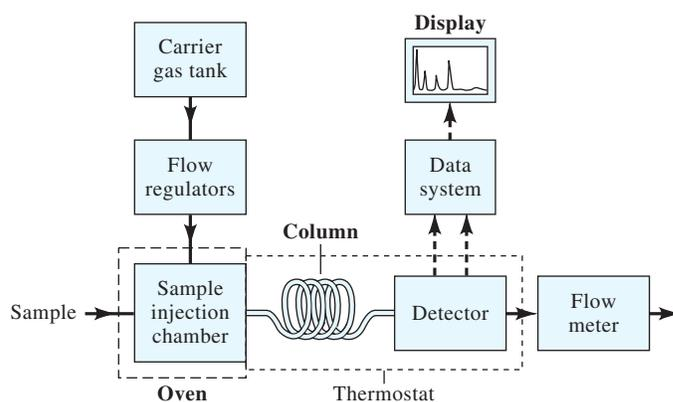
FIGURE 27-1 Block diagram of a typical gas chromatograph.
