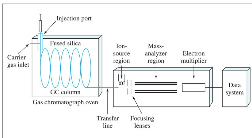
**FIGURE 27-15** Schematic of a typical capillary GC/MS system. The effluent from the GC is passed into the inlet of the mass spectrometer, where the molecules in the gas are fragmented, ionized, analyzed, and detected.
