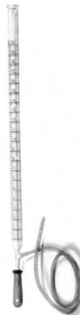
FIGURE 27-2 A soap-bubble flow meter. (Courtesy Agilent Technologies.)
