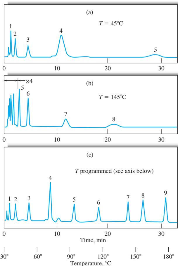
**FIGURE 27-8** Effect of temperature on gas chromatograms: (a) isothermal at 45°C, (b) isothermal at 145°C, and (c) programmed at 30–180°C. (From W. E. Harris and H. W. Habgood, *Programmed Temperature Gas Chromatography*, New York: Wiley, 1966, p. 10. Reprinted with permission.)
