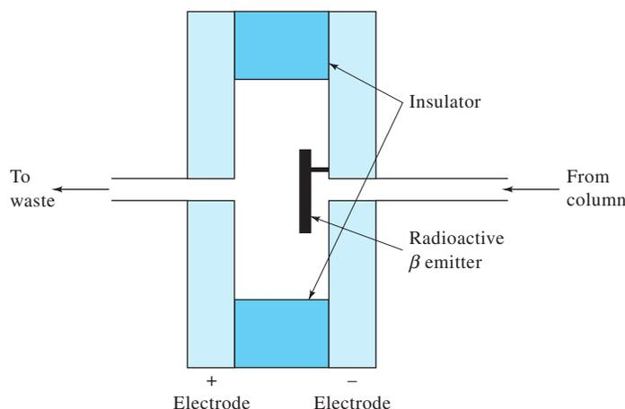
FIGURE 27-11 Schematic diagram of an ECD.
