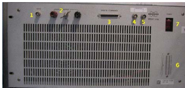
Figure 10.4 Great Amplifier Front View
