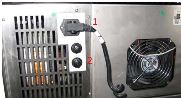
Figure 10.5 Back side view of the Great Amplifier showing the location of the fuses
