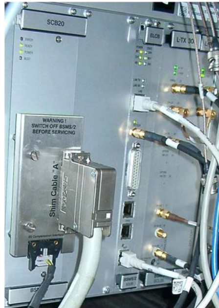
Figure 10.8 BSMS-2 to B0-2 Adaptor Board, mounted on the most right SCB20 Module
