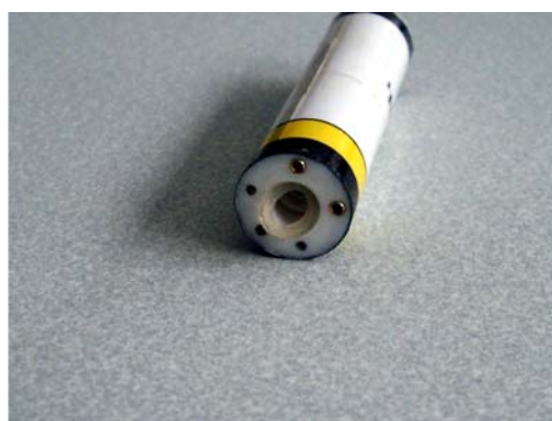
Figure 9.5 Bottom view showing silicon rubber sealing
