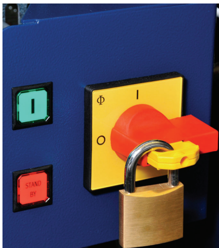
Fig. 13: System can be secured against unauthorized use by safety lock. Switch On of system is impossible when locked. All internal lines besides those marked by orange isolation are cut from electrical power supply. Generation of X-rays is impossible when system is locked.
