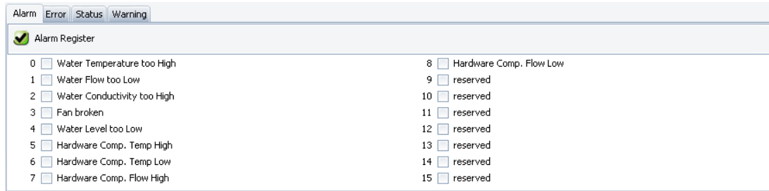
Figure 13.4: Alarm register for a water cooling unit
