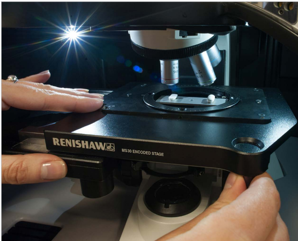
Renishaw's patented motorised stage uses encoders to keep track of its position, even when you move it manually.
