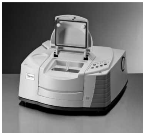
FIGURE 16-6 Photo of a basic, benchtop FTIR spectrometer suitable for student use. Spectra are recorded in a few seconds and displayed on a laptop computer. Software is available for controlling the instrument, collecting and processing data, and analyzing the results. An IR database is included for analysis and spectral interpretation. (Courtesy of Thermo Electron Corp., Madison, WI.)
