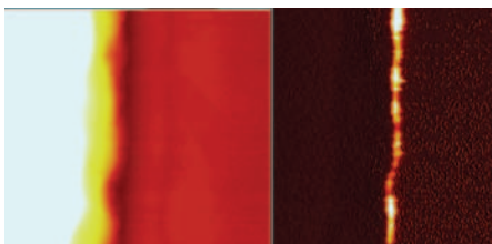
Figure 7. Topography (left) and simultaneously-obtained tunneling current image (right) at the transition from a field oxide to a 40nm thick gate oxide. At the transition the tunneling current is increased, which indicates thinning of the silicon oxide. 1µm scans, 0.5 pA current scale. Image courtesy A. Olbrich, Infineon, Munich, Germany.
