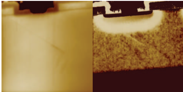
Figure 25. Topography (left) and resistance (right) scans of a cross-sectioned Si DMOS transistor. 1.2 \mu m scan courtesy IMEC, Belgium.
