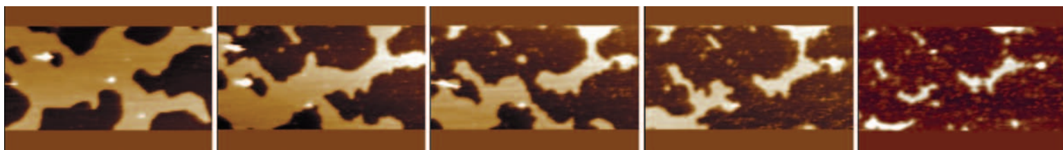
Figure 2. Action of PLA2 on a DMPC bilayer deposited on mica. 1\mu\text{m} \times 0.5\mu\text{m} scans.
