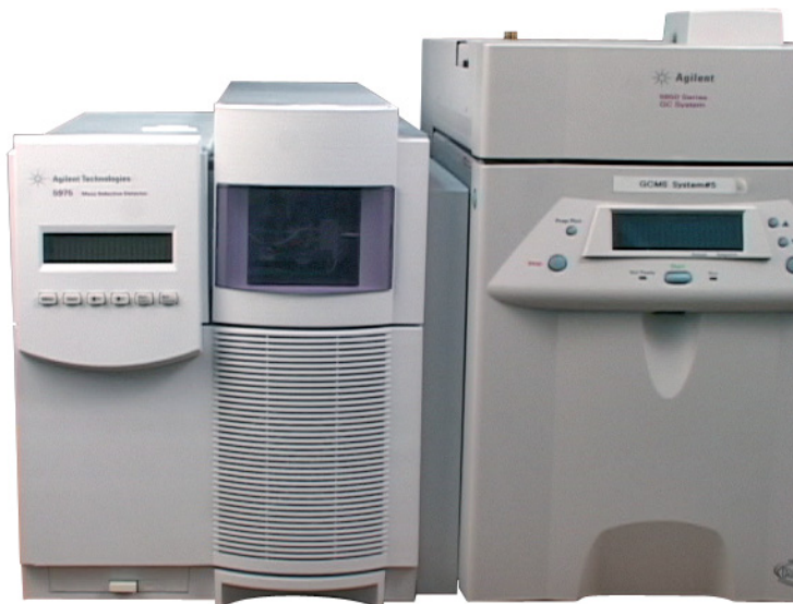
Figure 12 MSD and 6850 GC properly positioned
