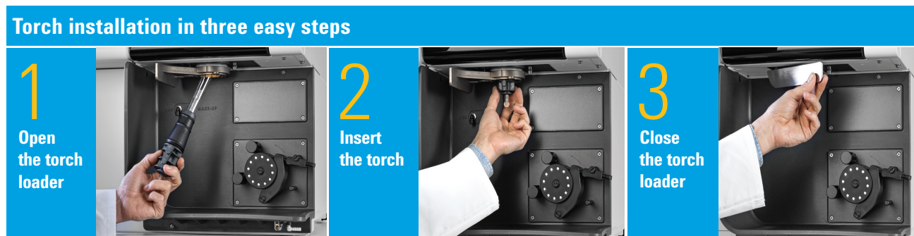
Figure 2. Sequence of 3-easy steps to load the torch into the instrument for fast start up and reproducible performance.
