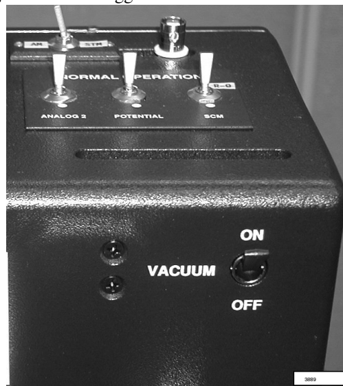
Figure 300.5a Toggle Switches on Dimension Electronics Box
