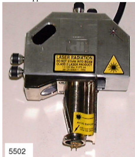
Figure 300.4a Application Module AFM Scanner
