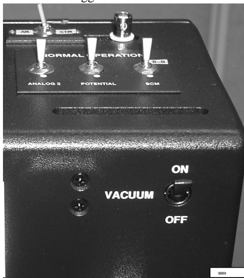
Figure 293.5a Toggle Switches on Dimension Electronics Box
